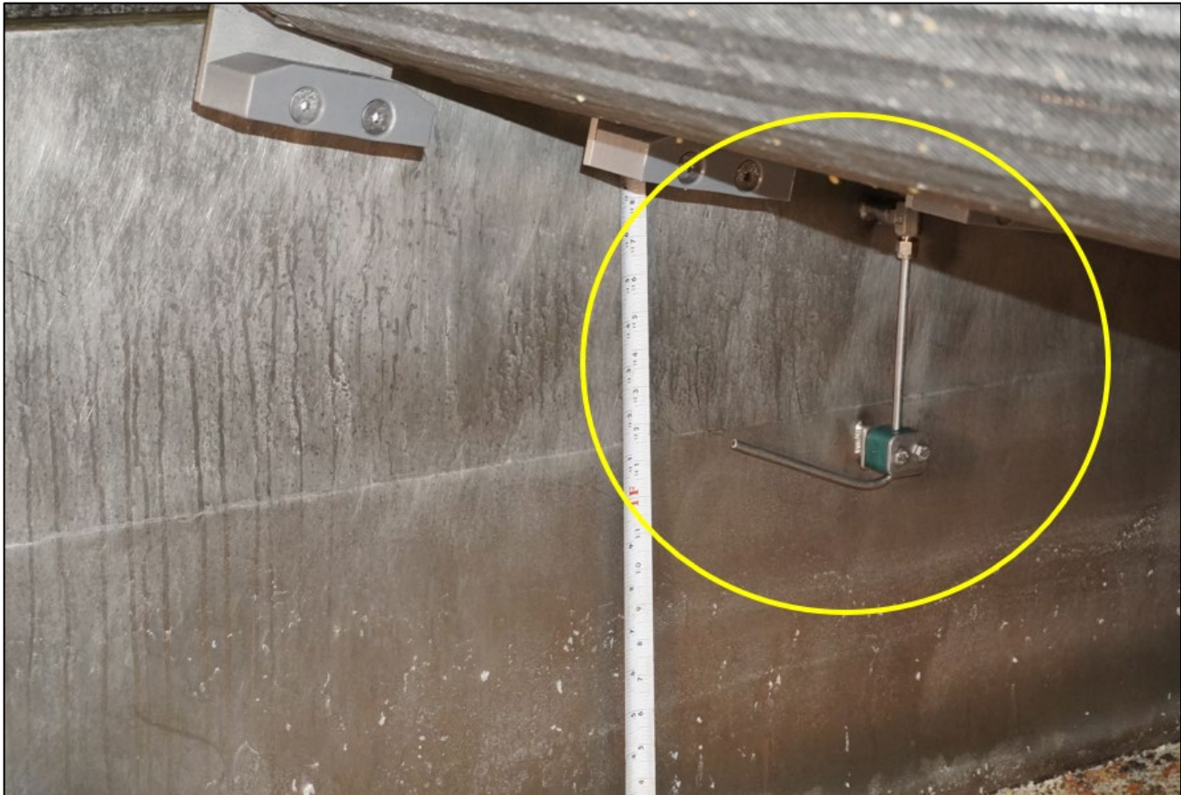
Figure 10. Immersion freezer bubbler tube, as found during the post-incident examination of the freezer. As designed, the tube should be pointing straight downward. (Credit: CSB)
