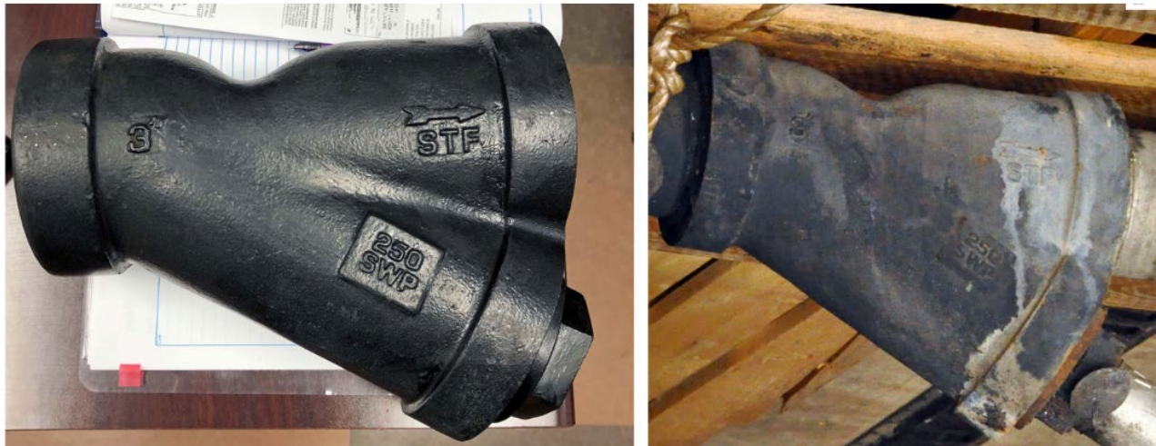
Figure 19. Exemplar Y-Strainer. The CSB purchased an exemplar y-strainer (left) using the inventory information available in KMCO’s warehouse. The image on the right shows the y-strainer involved in the incident. (Credit: CSB)
