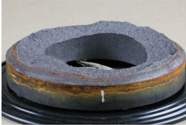
Figure 13. AW234 graphite nozzle fracture. (Credit: Wacker)
