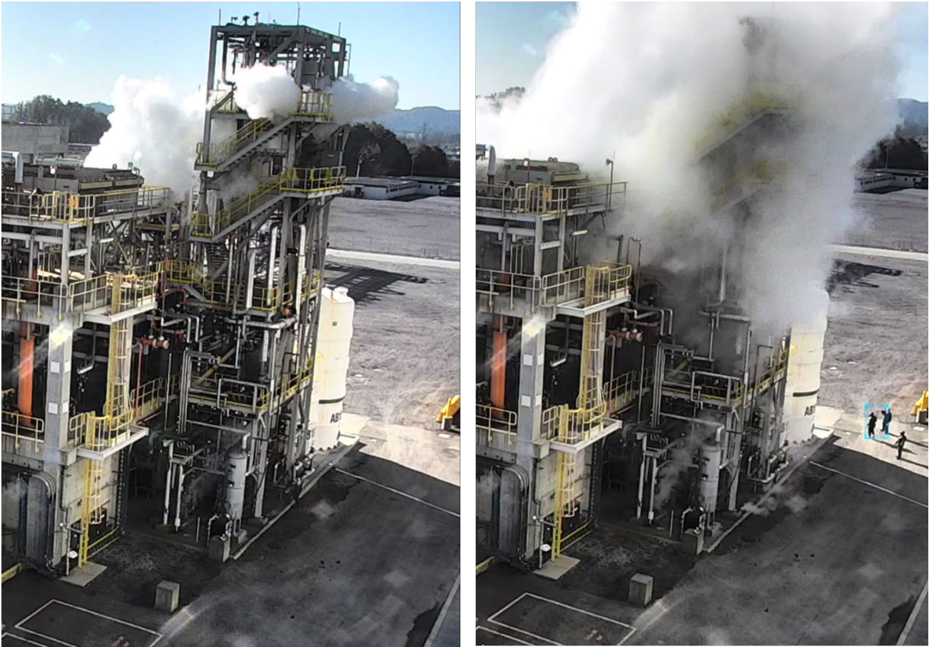
Figure 10. Image of HCl release at the time of release (left) and 15 seconds after release (right). (Credit: Wacker)
