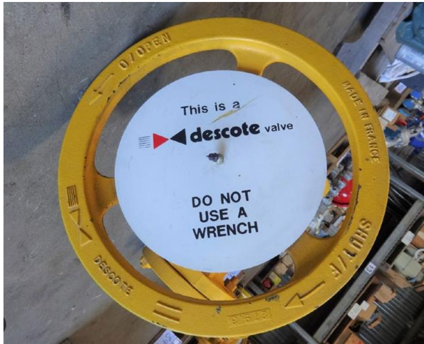
Figure 10. Photograph of a Descote valve’s warning sign to not use a wrench on the valve. (Credit: Steven Levy Enterprises [14])
