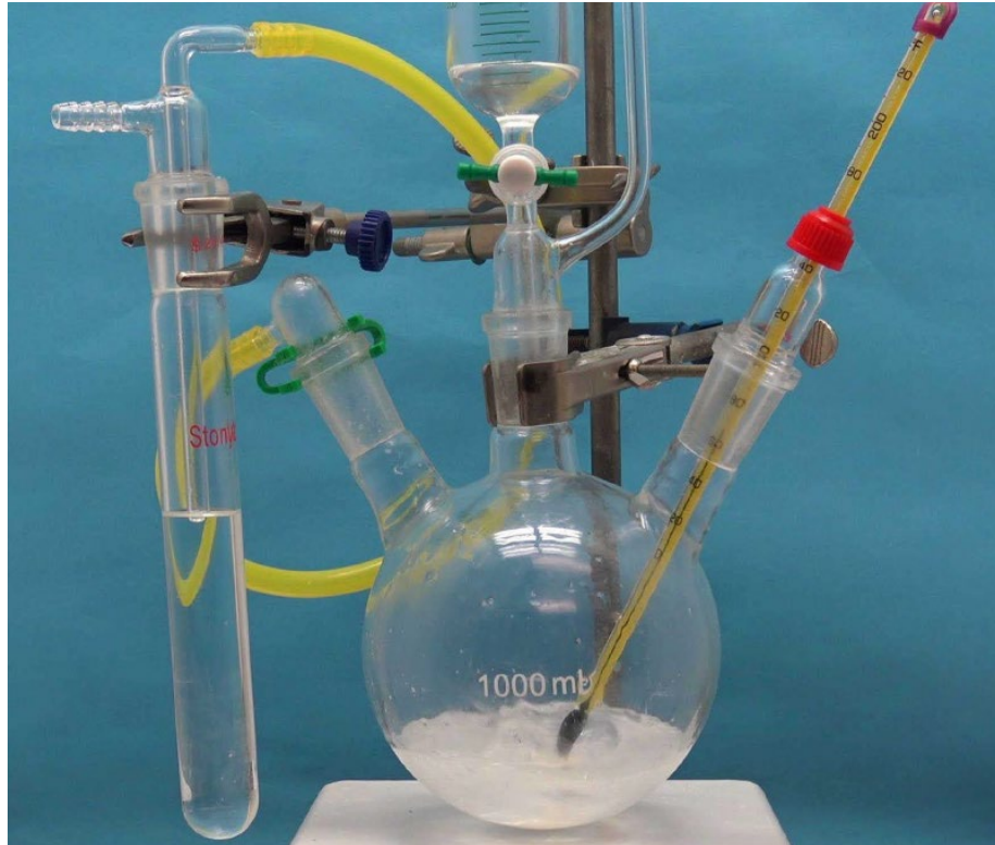
Figure C- 3. Closed system experimental setup – without Nitrogen and Flow Meter. (Credit: Crane)
