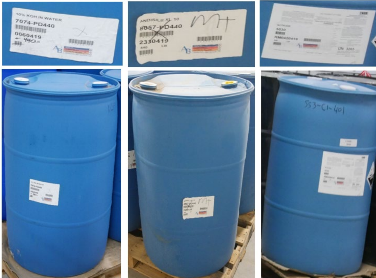
Figure 5. Three similar AB Specialty storage drums. From left to right: 10% KOH, XL 10, and Acticide. (Credit: CSB)
