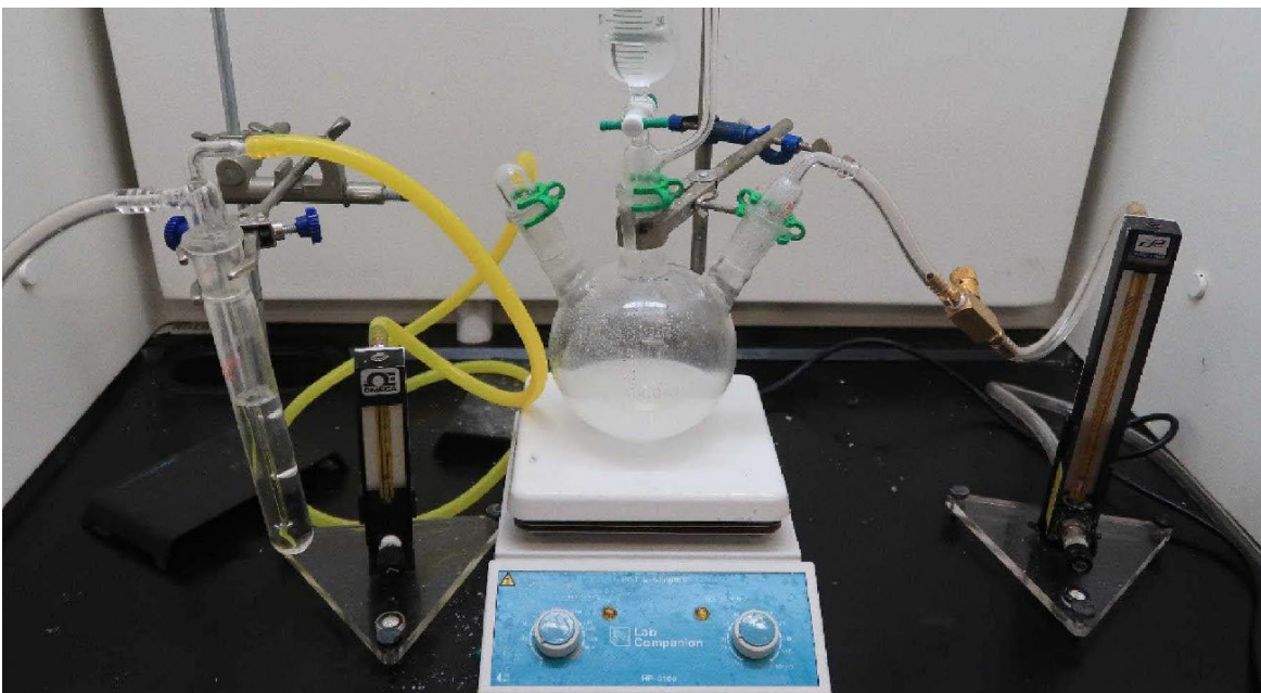
Figure C- 2. Closed system experimental setup – with Nitrogen and Flow Meter. (Credit: Crane)
