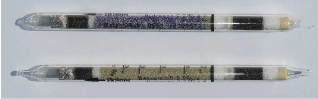
Figure C- 6. Hydrogen Dräger-Tube used to qualify hydrogen gas generation from o-TD-KOHa test (above) compared with sealed, unused Dräger-Tube (below). (Credit: Crane)
