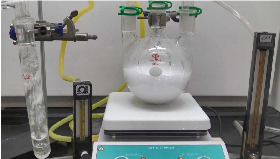
Figure C- 8. Photograph of TD-KOH test a few seconds before joint was blown off due to substantial gas generation. (Credit: Crane)
