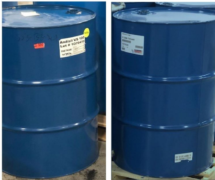
Figure 10. Two chemicals in similar drums involved in previous near-miss incident. (Credit: AB Specialty)
