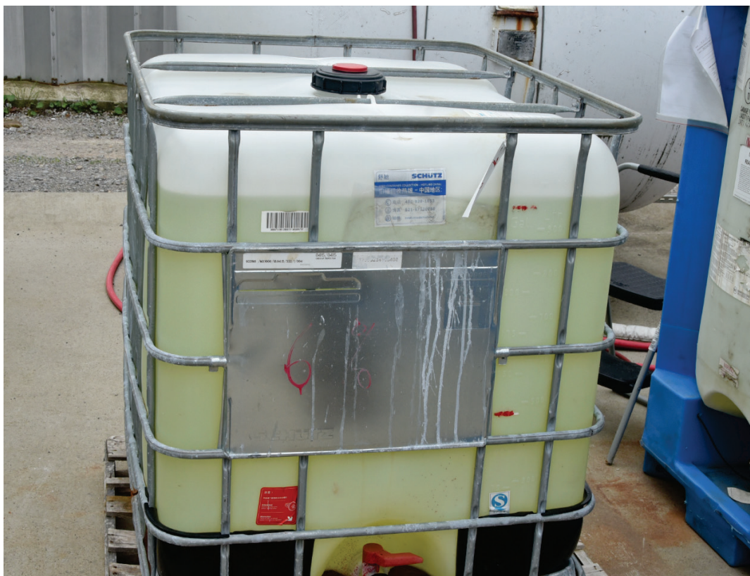
Figure 4. Sodium Hypochlorite Tote. This picture shows one of the totes at MRR that contained sodium hypochlorite. (Credit: CSB).
