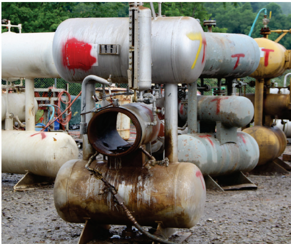
Figure 16. MP Odorizer Vessel That Exploded. This photo shows the MP odorizer that exploded on June 20, 2017. The back portion of middle chamber ruptured (see also Figure 17) and the front threaded section blew off. The aluminum tray and mechanical parts that were inside the middle chamber were expelled from the MP during the event. (Credit: SPSI).
