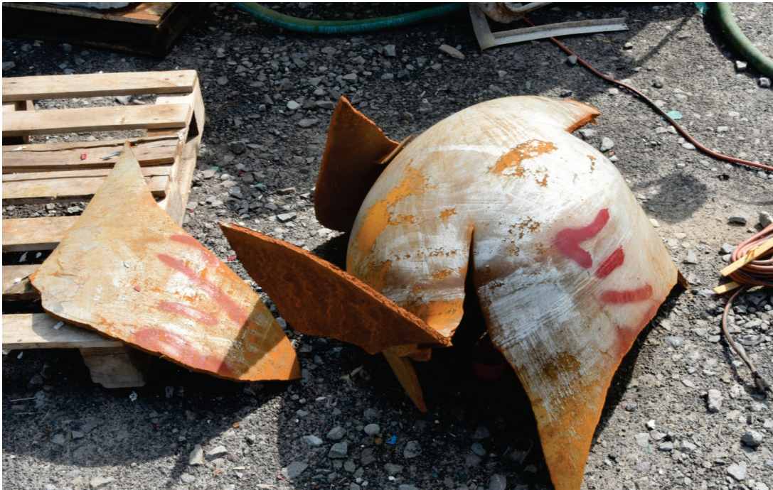
Figure 11. MP Odorizer Fragment from May 24, 2017, Explosion. This photo shows a portion of the top chamber of the MP odorizer after the May 24, 2017, explosion. (Credit: CSB).
