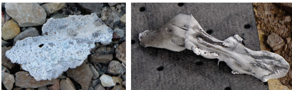
Figure 21. Aluminum Parts. The picture on the left shows an aluminum part from the MP odorizer involved in the May 24, 2017, incident that appears to have general corrosion. The photo on the right shows an aluminum part from the MP odorizer involved in the June 20, 2017, incident that appears to show signs of melting from heat. (Credit: MRR (left), SPSI (right)).
