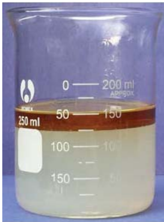
Figure 16. Photograph of Immiscible Oil Layer on Top of Water. This photograph shows how oil forms an immiscible liquid layer on top of water similar to how a turpentine layer might appear inside the foul condensate tank. Photograph: CSB.
