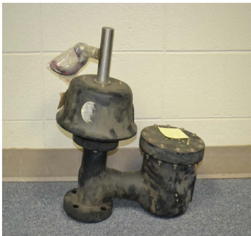
Figure 15. Photograph of a Spare Pressure Vacuum Breaker for the CNGC System at the DeRidder Mill. If the foul condensate tank experiences high-pressure (six-inches of water), the left-hand portion of the pressure vacuum breaker opens and releases vapor to the atmosphere. If the tank experiences low-pressure (minus six-inches of water), the portion of the pressure vacuum breaker extending to the right will open and pull air into the tank. b Photograph: CSB.
