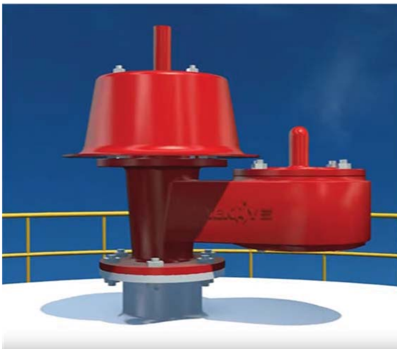
Figure 23. Image of a Pressure Vacuum Breaker. If the vessel experiences an over pressure event, the top portion of the pressure vacuum breaker releases to the atmosphere. If the vessel experiences an under pressure event, the portion of the pressure vacuum breaker extending to the right will pull air into the vessel. Photograph: Finekay [12].
