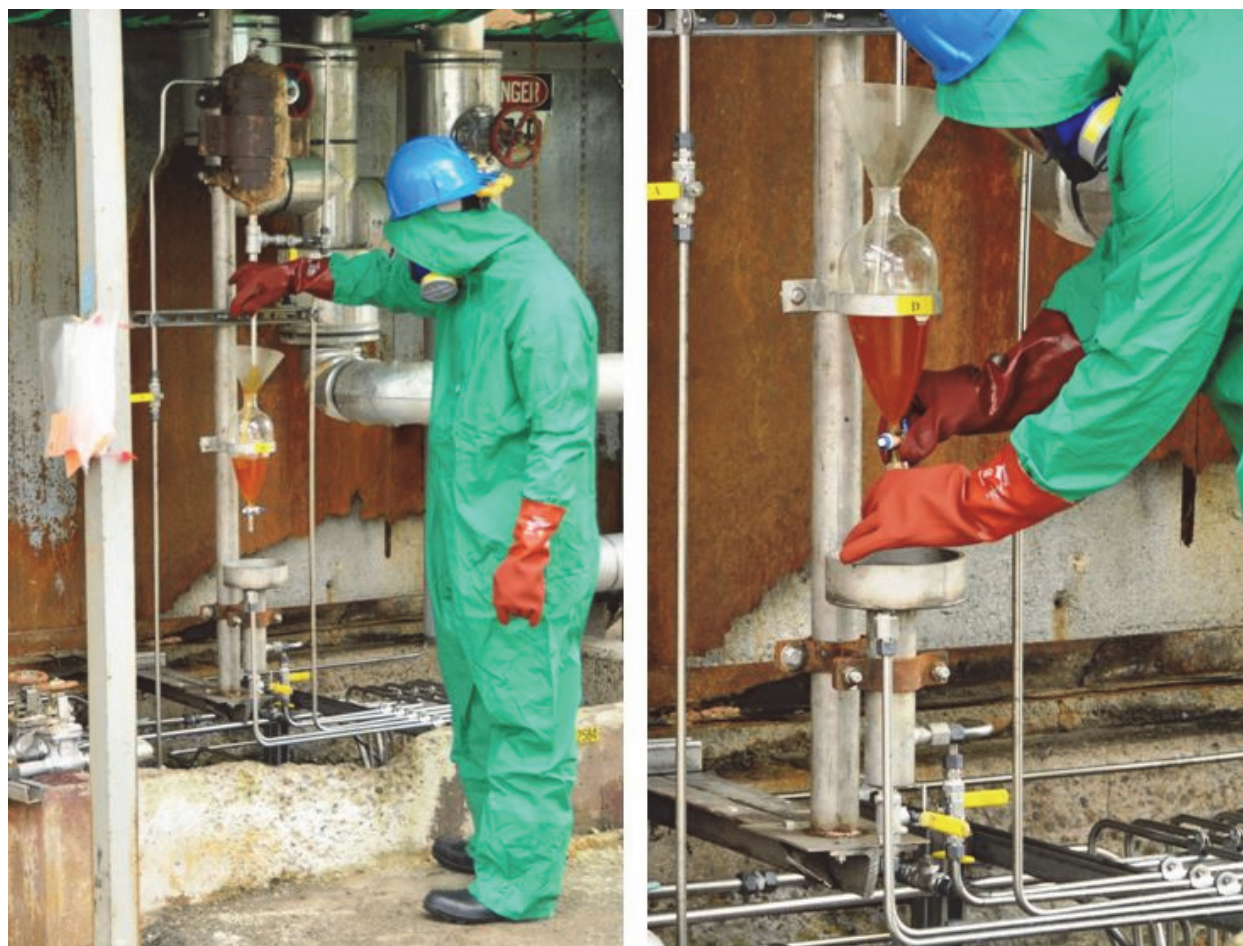
Figure 7. Photos of an operator at the Tesoro Martinez refinery taking a sulfuric acid sample. These photos were taken following the February 12, 2014 incident with the new PPE requirements in place. Tesoro’s sulfuric acid sampling system requires two separate one-hour waiting periods to allow hydrocarbons to vent to the atmosphere. In addition to potential liquid acid exposure, the sampling process exposes the operator to hydrocarbon vapor, and sulfuric acid vapor. Following the incident, Tesoro upgraded the PPE requirements to include a full-face respirator and a full-body acid suit.
