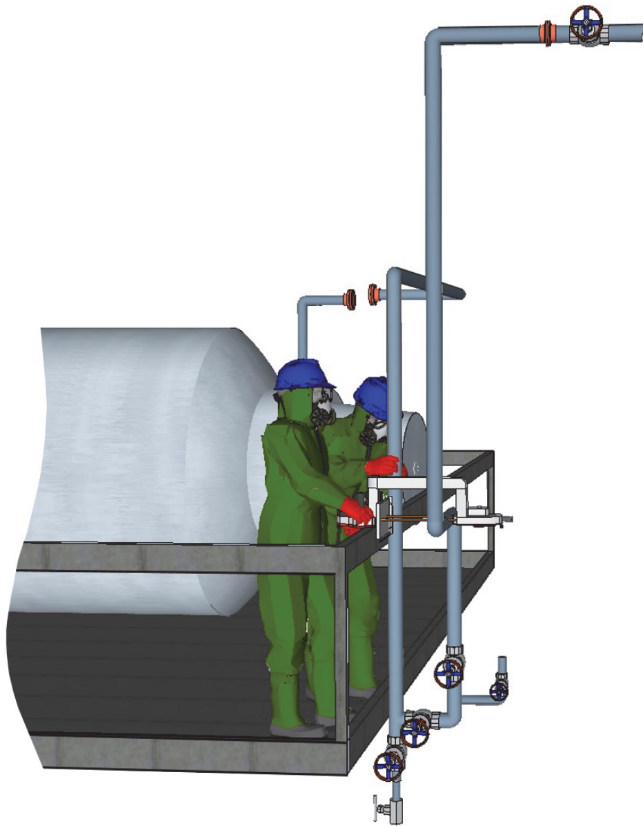
Figure 12. CSB depiction of the workers cutting the 1-inch butane piping just prior to the sulfuric acid spray incident on March 10, 2014.
