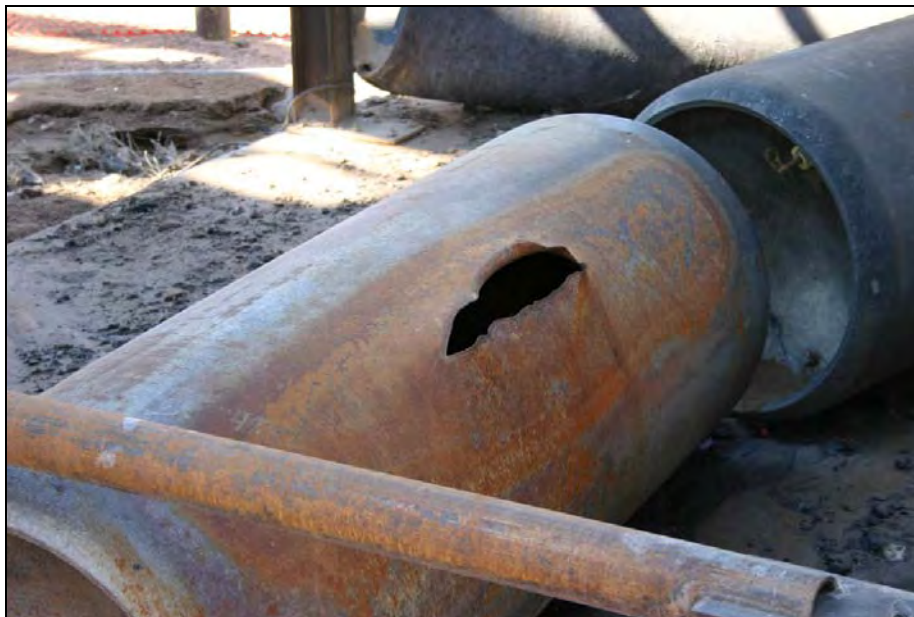
Figure 13. Ruptured one-ton chlorine container
