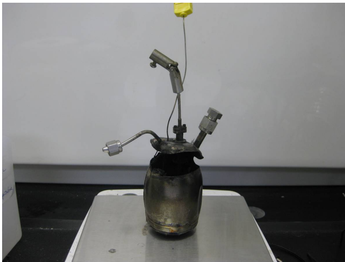
Figure 16. Burst VSP2 Test Cell.
