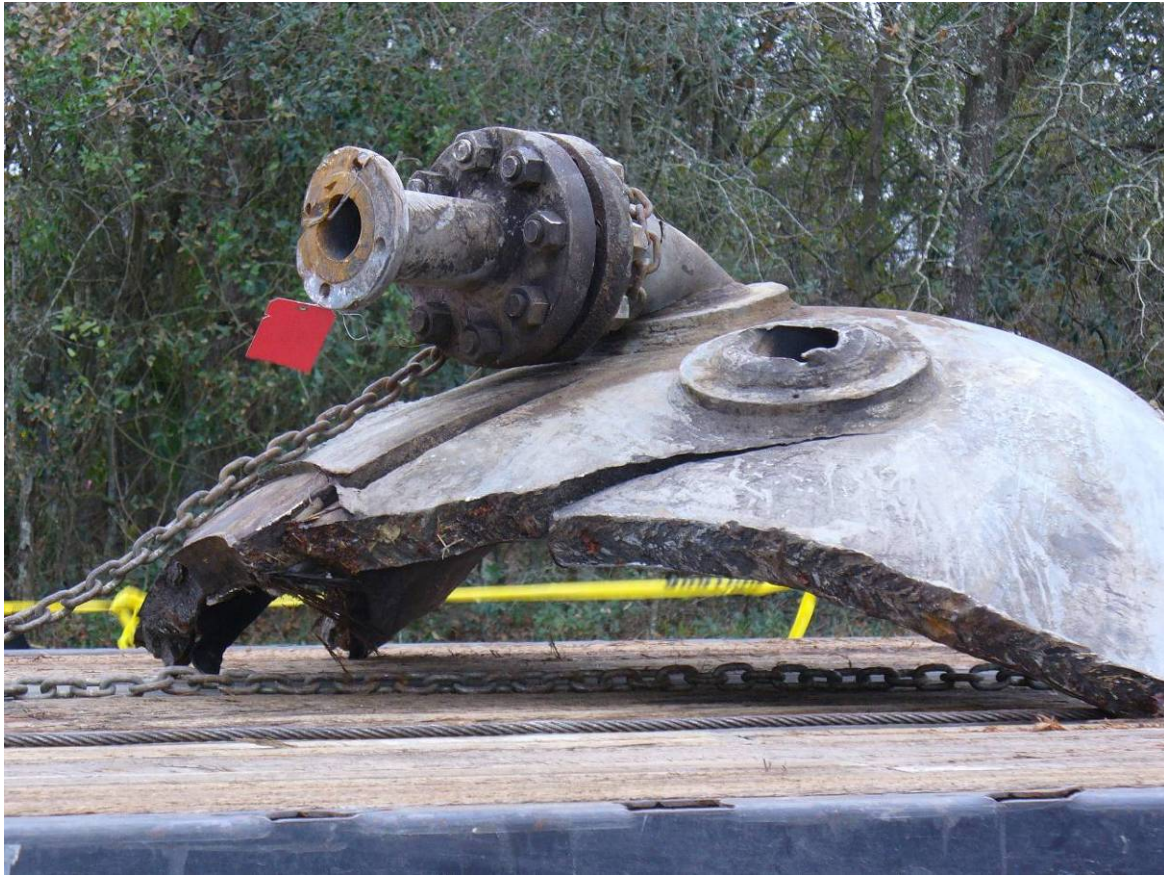
Figure 5. Portion of the 3-inch-thick reactor.
