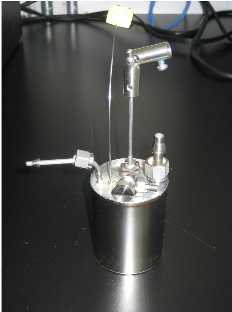
Figure 15. New VSP2 Test Cell.
