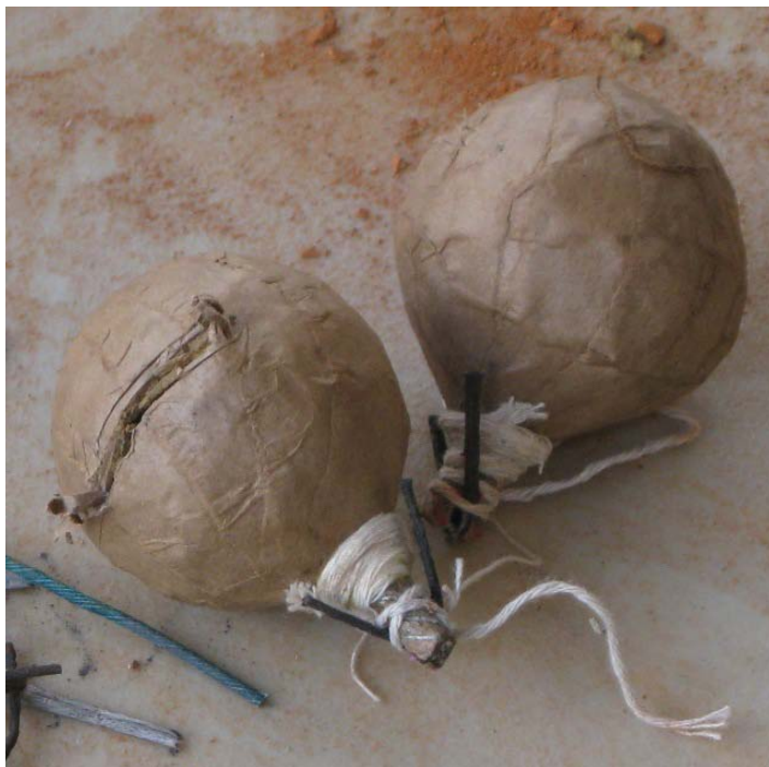
Figure 7. Slit aerial shell from DEI's first destruction
