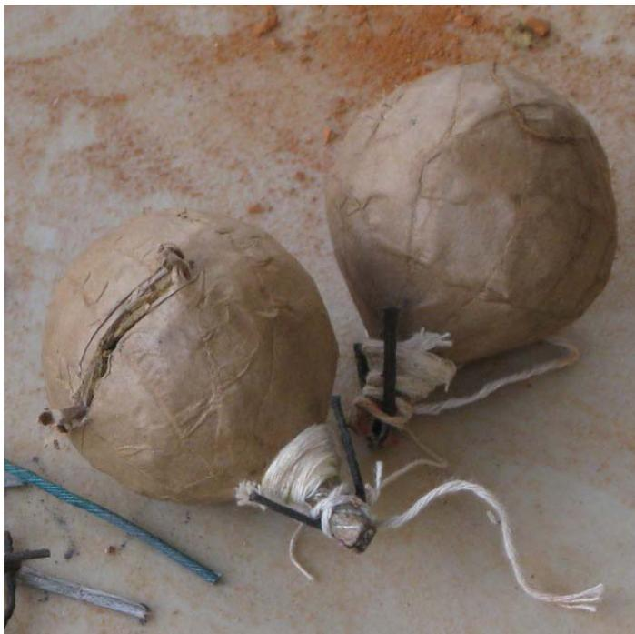
**Figure 7. Slit aerial shell from DEI's first destruction**
