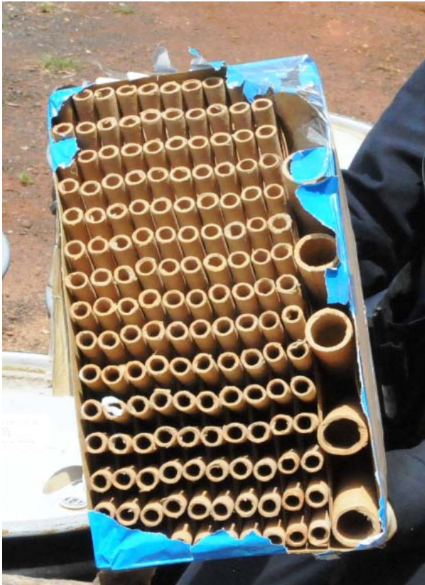
Figure 12. Sky Festival cake firework (from the primary seizure) contains 150 small tubes and 6 large tubes; large tubes located on the right side of the box were being disassembled on the day of the incident.
