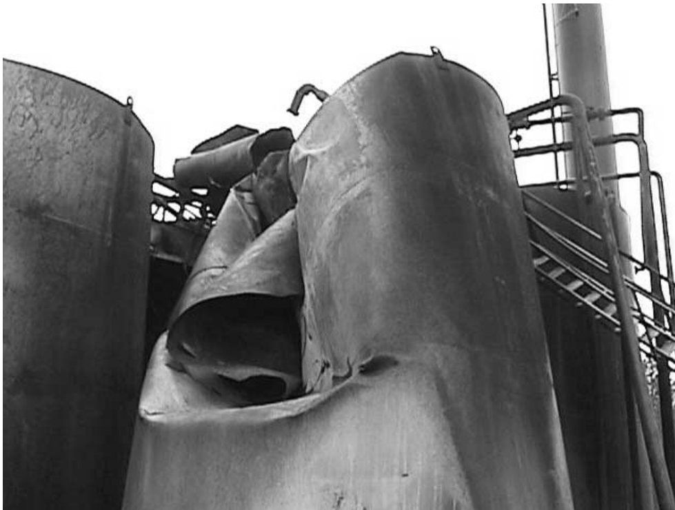
Figure 8. Damaged Water Storage Tank with Fragment of Third-Stage Separator
