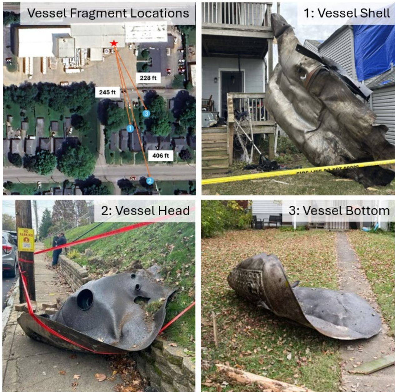
Figure 6. Locations of Batch Reactor Six debris scattered throughout the surrounding neighborhood. (Credit: Map: Google Earth with annotations by CSB; Photo 1: Dylan Lovan, Associated Press via Louisville Public Media [10]; Photo 2: WDRB News [11]; Photo 3: Louisville Courier Journal [12])
