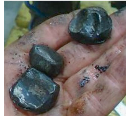
Figure 1. Damaged Pump Bearings. (Credit: Pemex)
