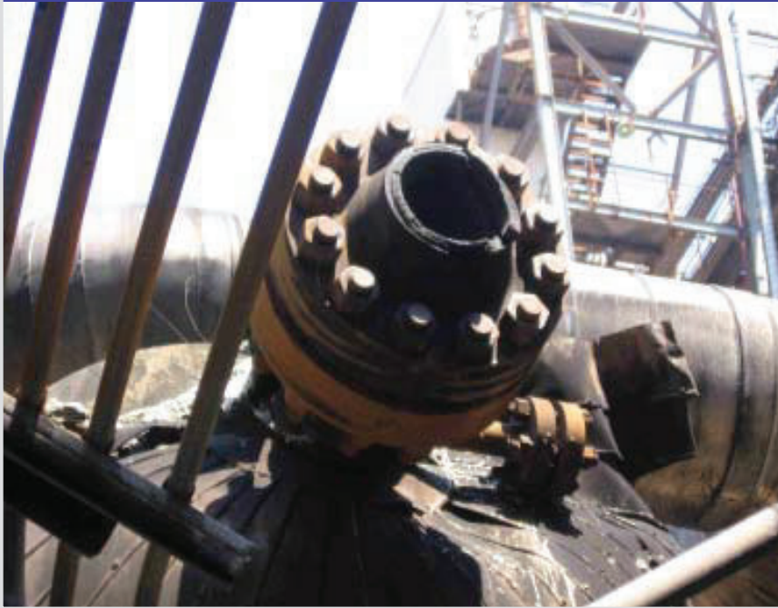
Figure 4. Ruptured 8-inch carbon steel pipe elbow pieces recovered after the fire
