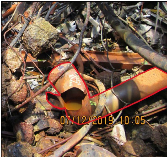
Figure 22. The ruptured elbow as found in the PES alkylation unit after the incident (left, outlined in red) and the same rupture during metallurgical testing (right).
