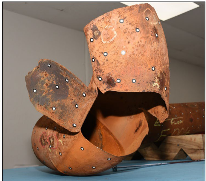
Figure 22. The ruptured elbow as found in the PES alkylation unit after the incident (left, outlined in red) and the same rupture during metallurgical testing (right).
