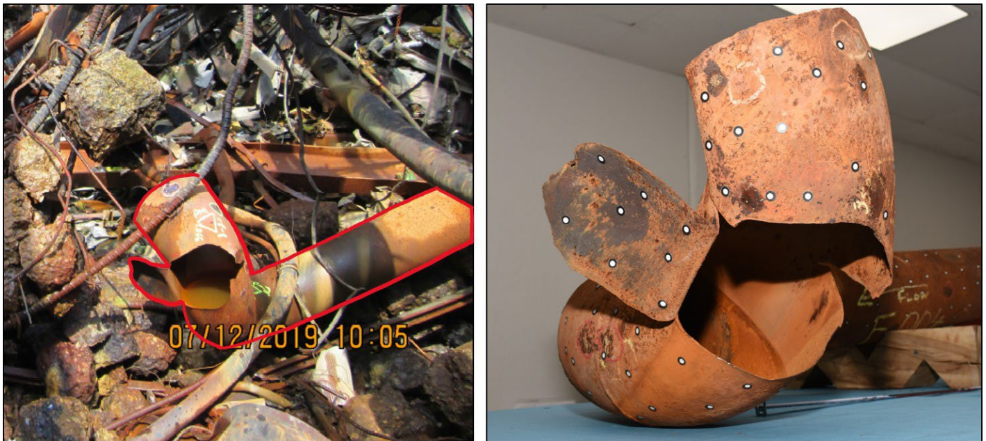
Figure 15. The ruptured elbow as found in the PES alkylation unit after the incident (left, outlined in red) and the same rupture during metallurgical testing (right).
