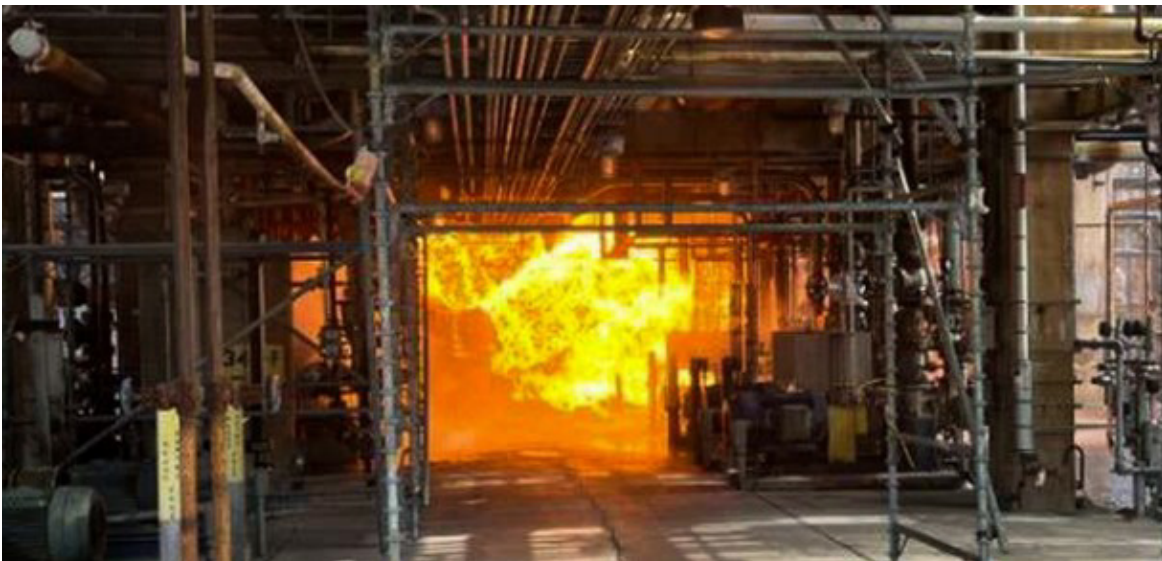
Figure 14. Fire from breached piping. (Credit: Marathon)
