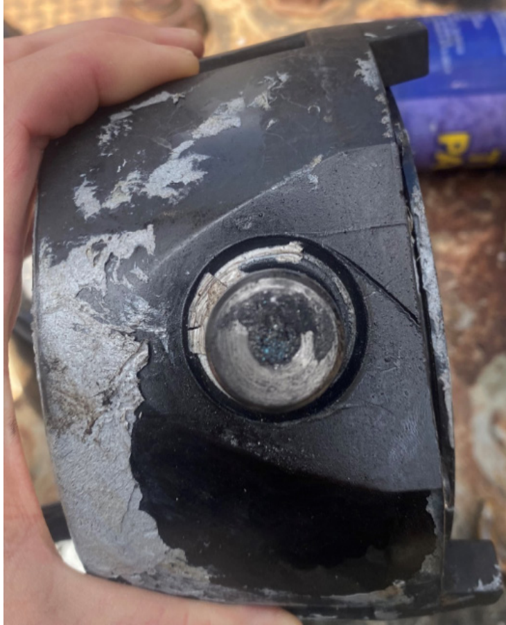
Figure 2. Pressure gauge involved in the incident. (Credit: Marathon)
