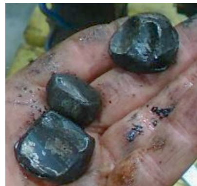
Figure 1. Damaged Pump Bearings. (Credit: Pemex)
