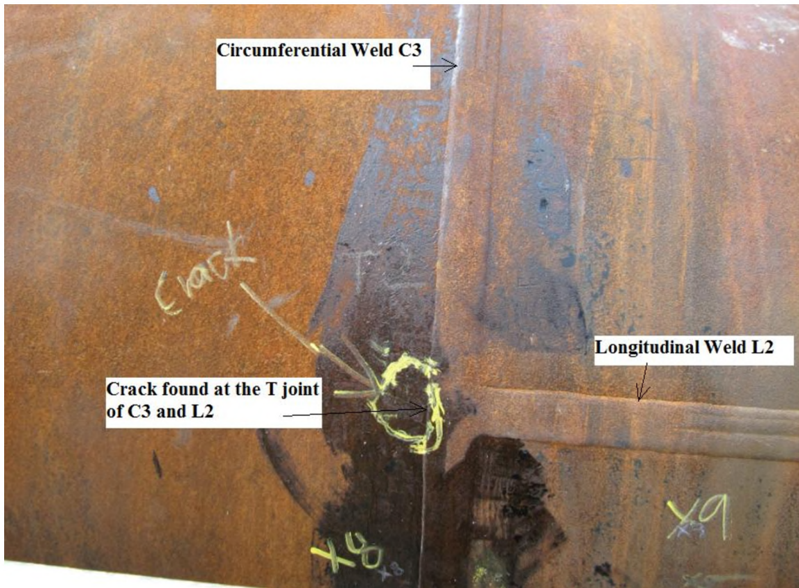
T joint of Circumferential weld C3 and Longitudinal L2
