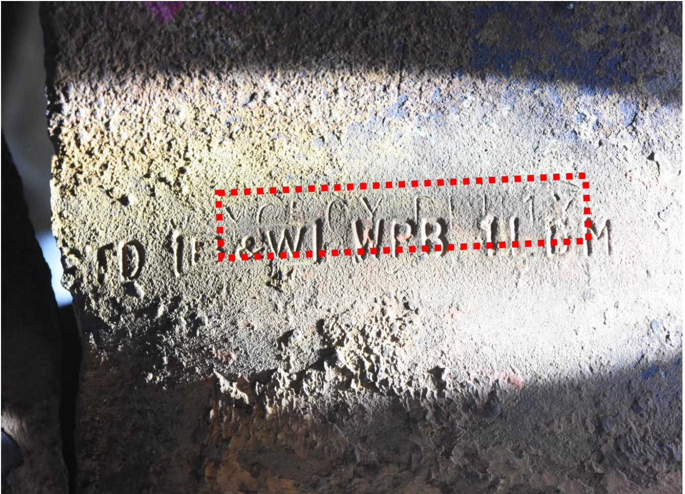
Figure 16. Photo of specification stamps on the failed elbow. “YOLOY,” highlighted with red, is faintly visible behind the “WPB” stamp.
