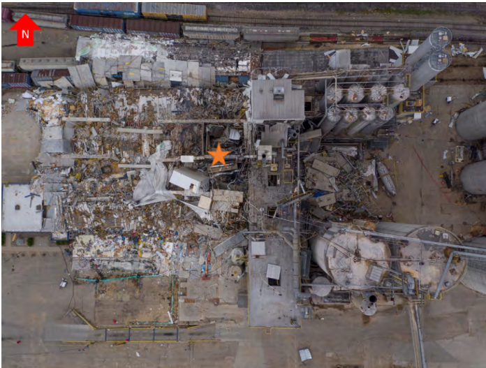
Figure 17. Approximate location (gold star) of the second explosion after the collapse of the mill buildings.
