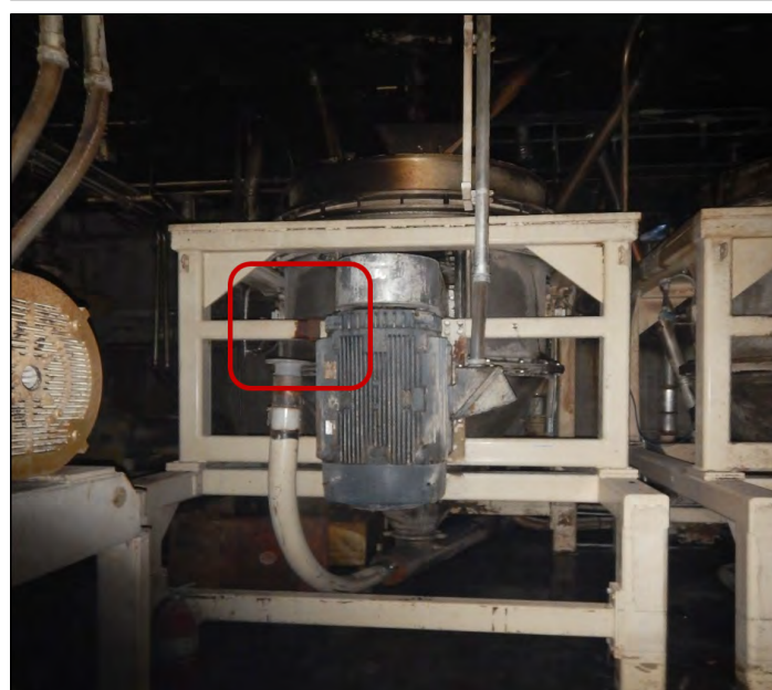
Figure 12. The Superintendent saw the filter from the south gap mill air intake line flying in the air and a three- to four-foot flame shooting out from the same line (red box, top image). The post-incident photograph (bottom) shows the filter missing (red box).
