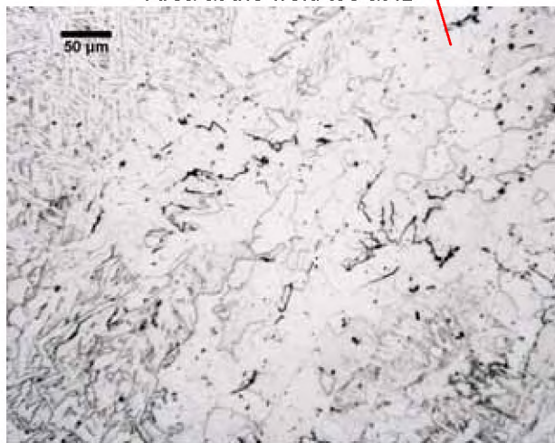
Weld metal near ID. Etched
