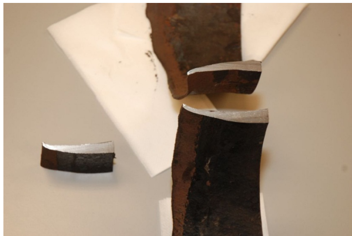
Figure 30. Images showing sectioning of the SER 34 fracture surface for metallographic and quantitative chemical analyses in August 2010.
