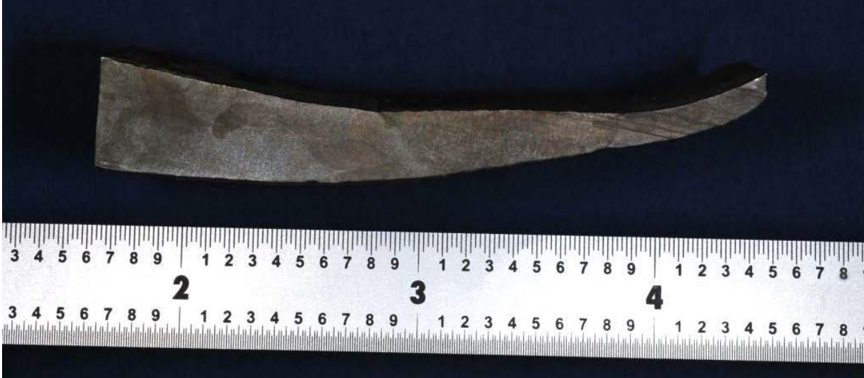
Figure 31. Image of the metallographic longitudinal cross-section specimen from the 6-o'clock location on SER 34, showing wall thickness loss at the ID surface through the weld metal and base metal of the straight segment.
