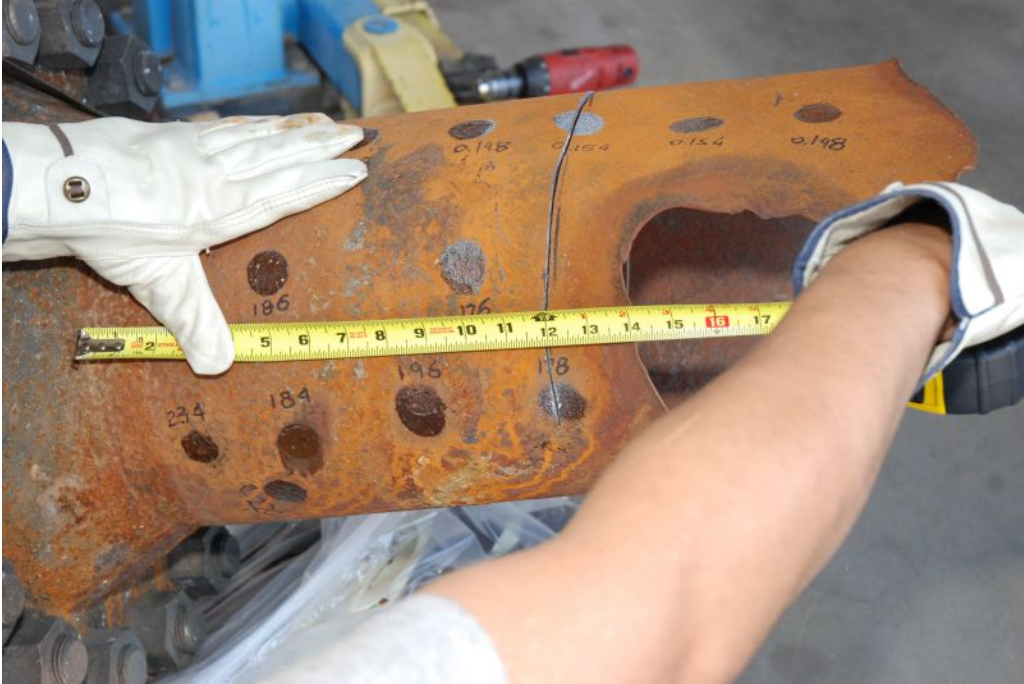
Figure 27. The fractured end of SER 35 during sectioning in August 2010.
