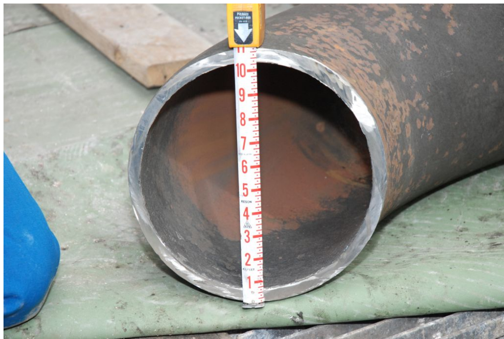
Figure 20. Images of the "SER 34" ruptured segment after sectioning and removal in March 2010.
