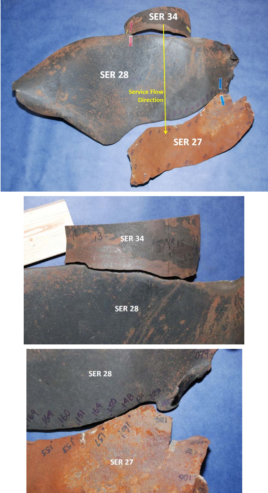
Figure 35. Images showing the in-service locations of SER 34, SER 28, and SER 27 based on alignment of fracture surface features.
