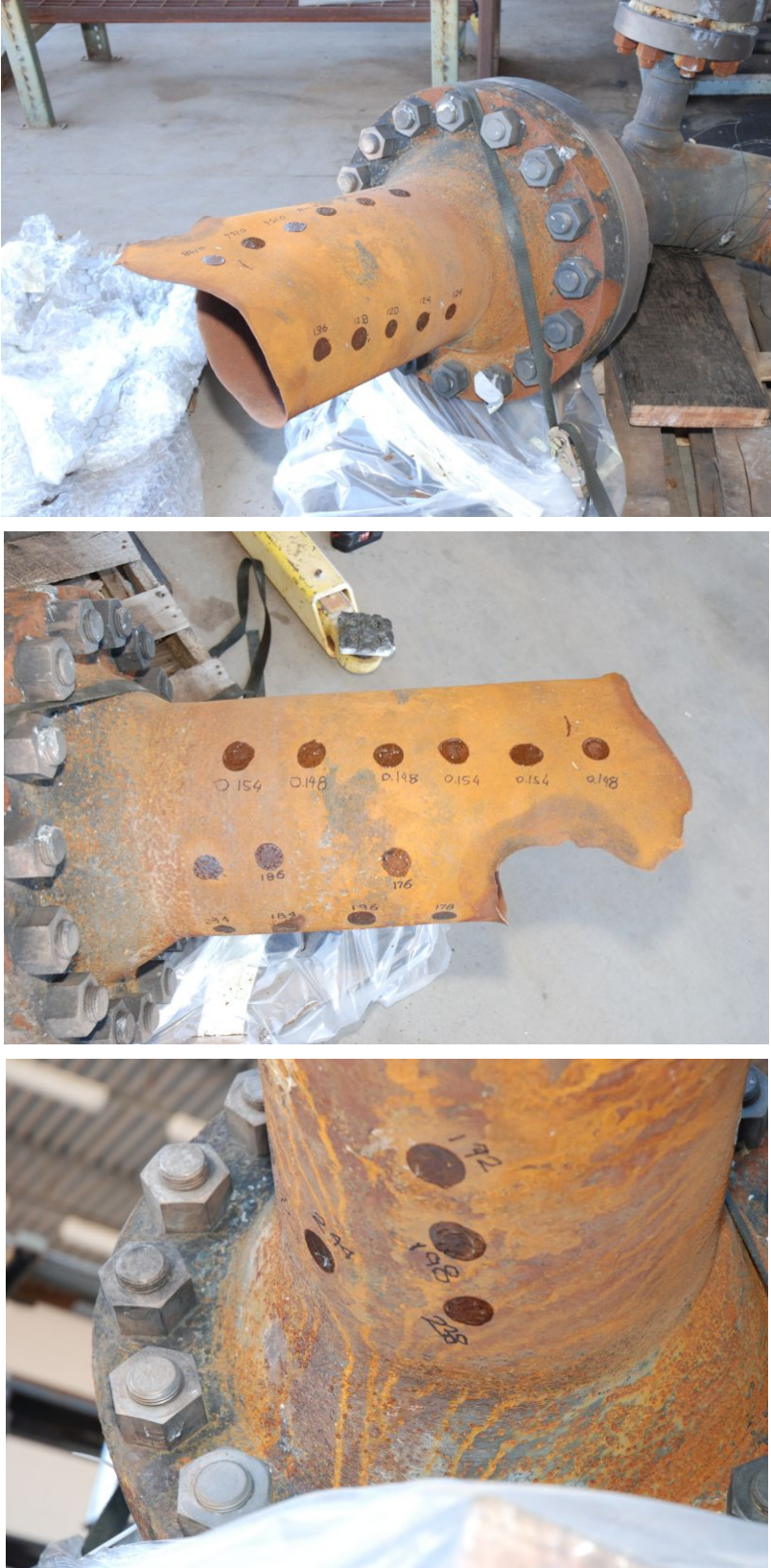
Figure 26. Images showing UT measurements taken on the SER 35 segment in August 2010.
