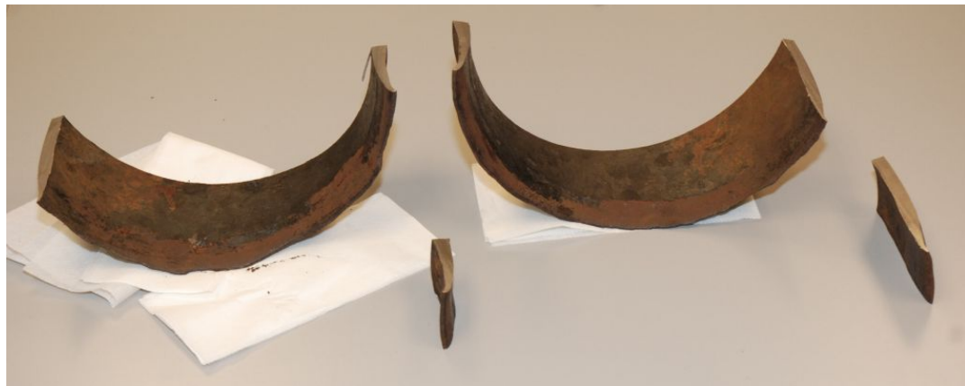
Figure 29. Image showing quantitative chemical analysis samples being sectioned from the 10-inch pipe and flange on SER 35 (circled) in August 2010.
