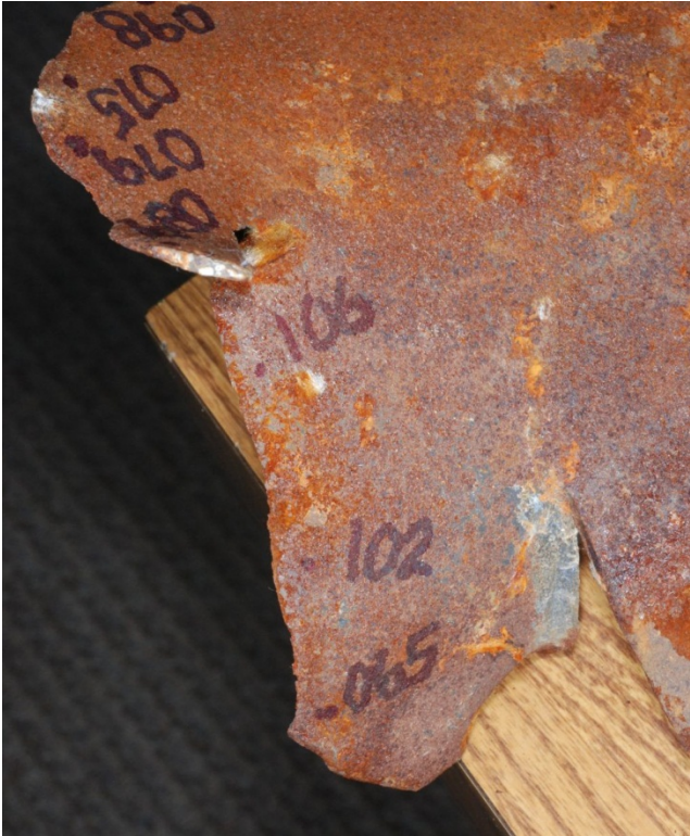
Figure 33. Images of SER 27 showing the results of wall thickness measurements.
