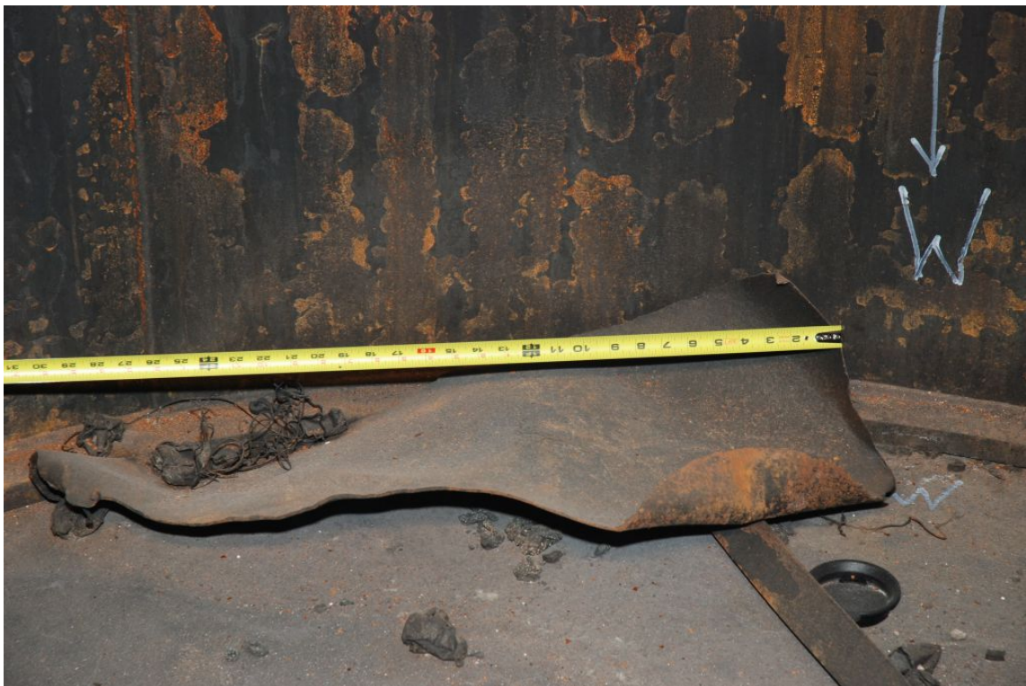
Figure 25. Image of the "SER 28" item as-observed inside the reactor skirt in March 2010.
