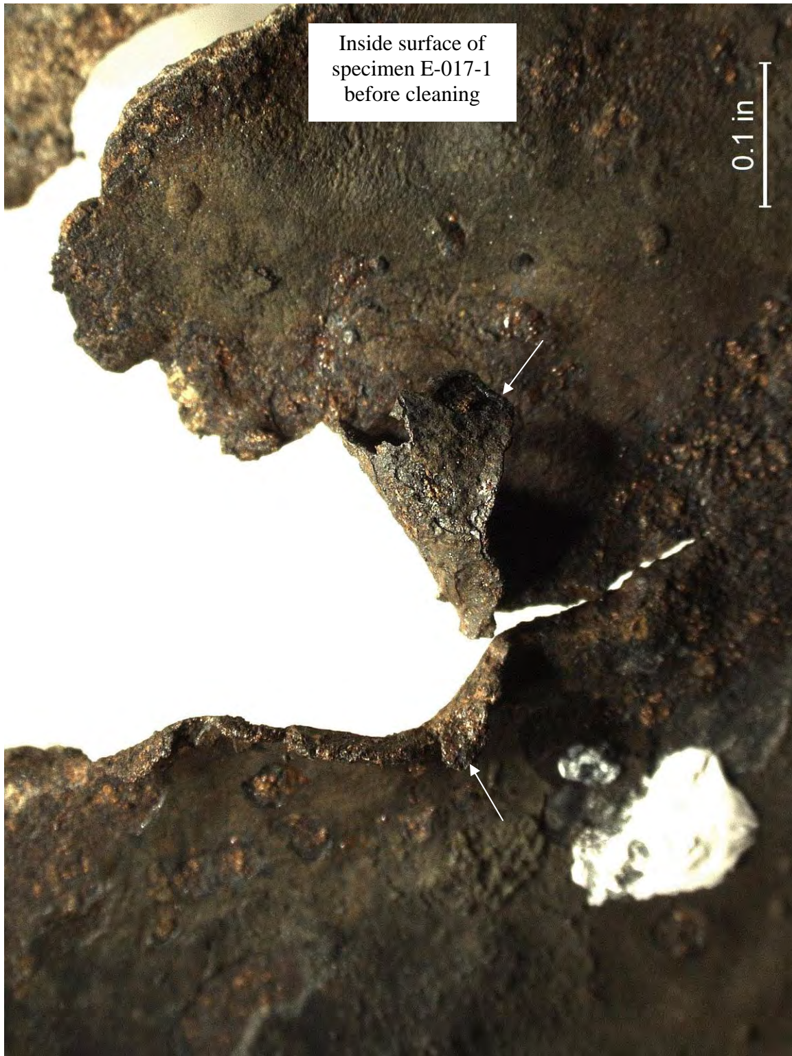
Figure 17 Macrograph of the inside surface of specimen E-017-1 taken from the region indicated in Figure 8 before cleaning. Deformation of the specimen edge, indicated by arrows, was consistent with mechanical force applied from the outside.
