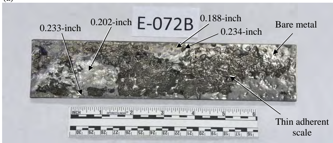
Figure 33 Photographs of the inside surface of cleaned specimens sectioned from the 12-inch 4-sidecut samples.
