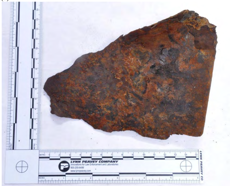
Figure 11 Fragment E-014 recovered from the ground beneath the rupture.
