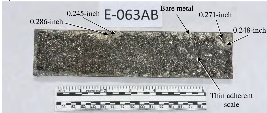
Figure 32 Photographs of the inside surface of cleaned specimens sectioned from the 12-inch 4-sidecut samples.
