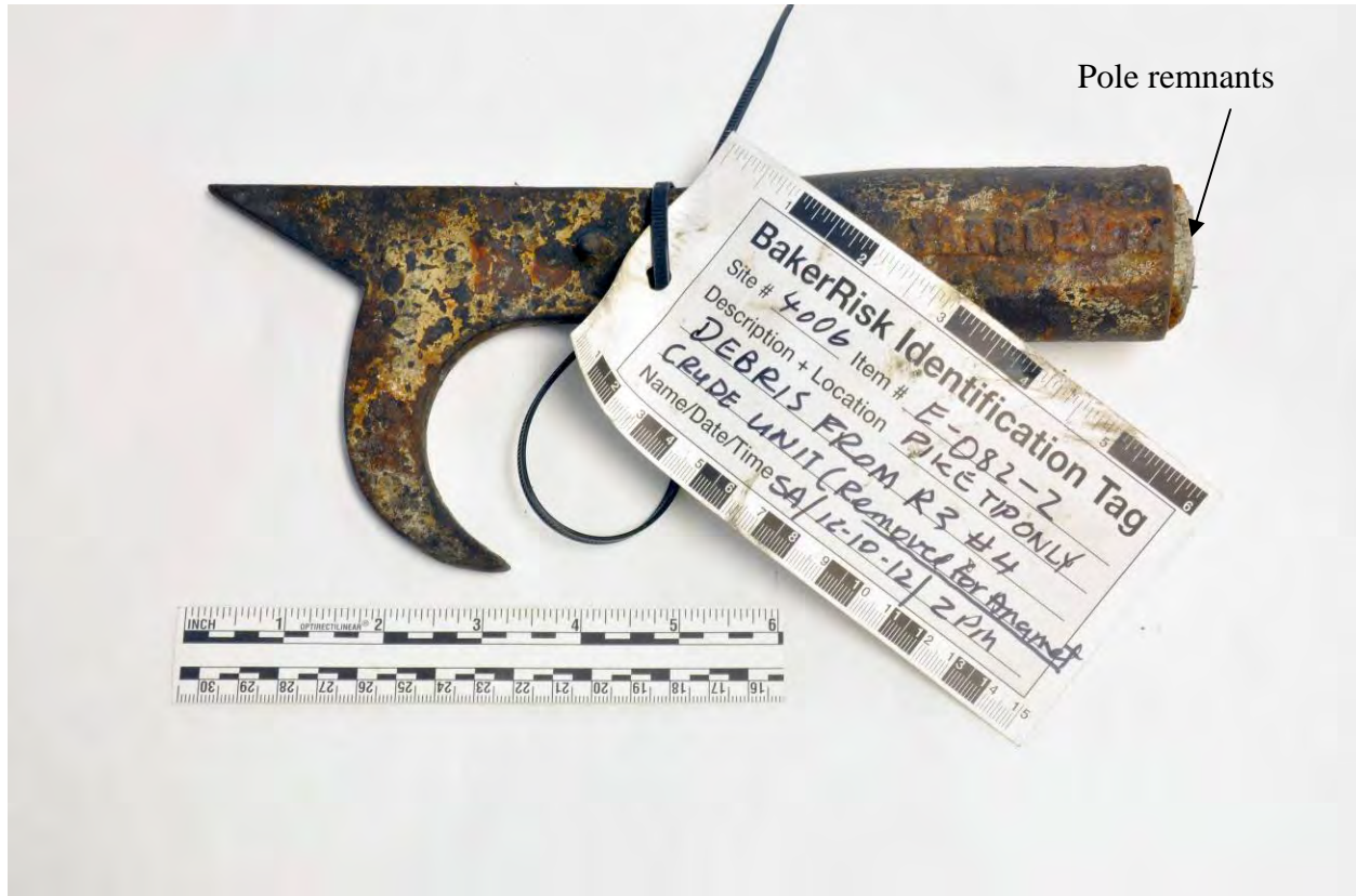
Figure 20 Photograph of pike pole head, sample E-082-2, recovered from the site of the ruptured 4-sidecut. The glass fiber reinforced polymer pole was absent except for the indicated remnants.
