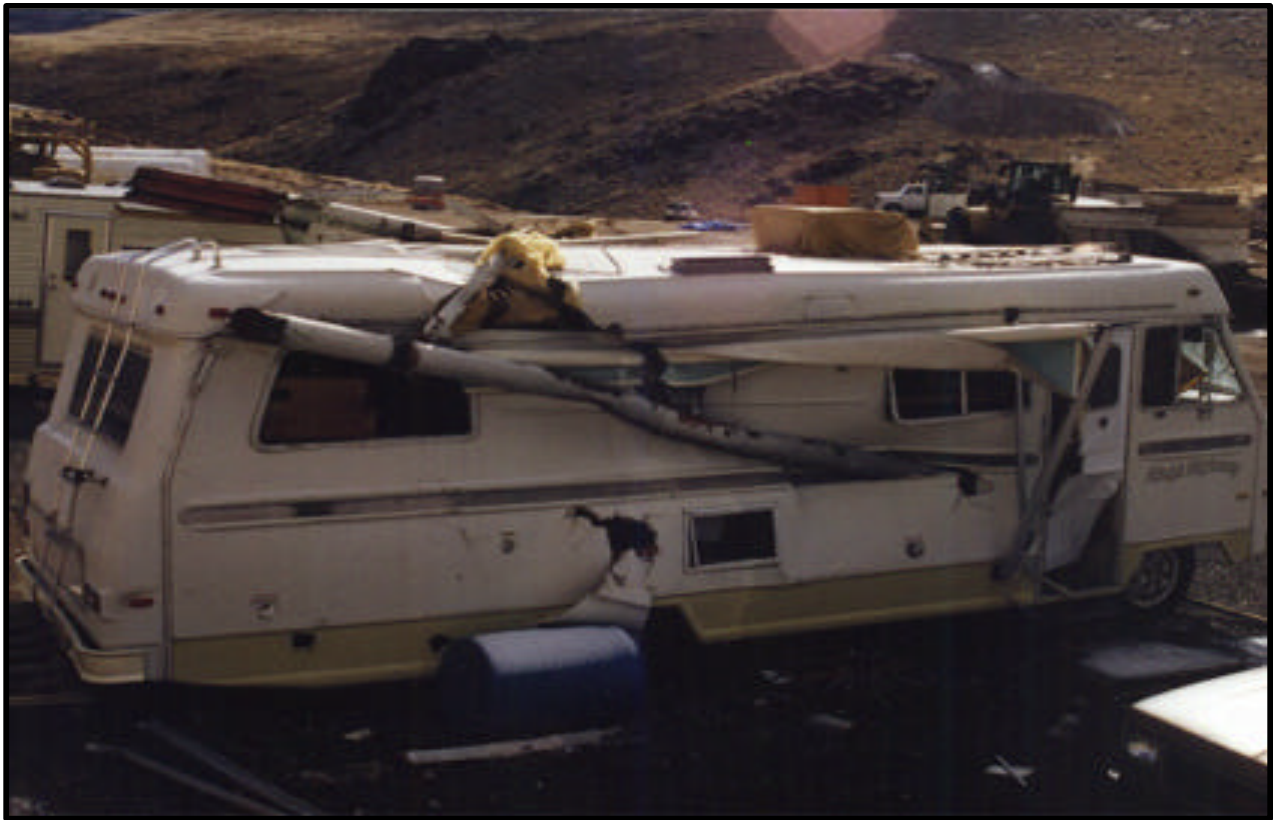
Figure 10. Mobile Home Hit by Legs of Tank and Cross Bracing
