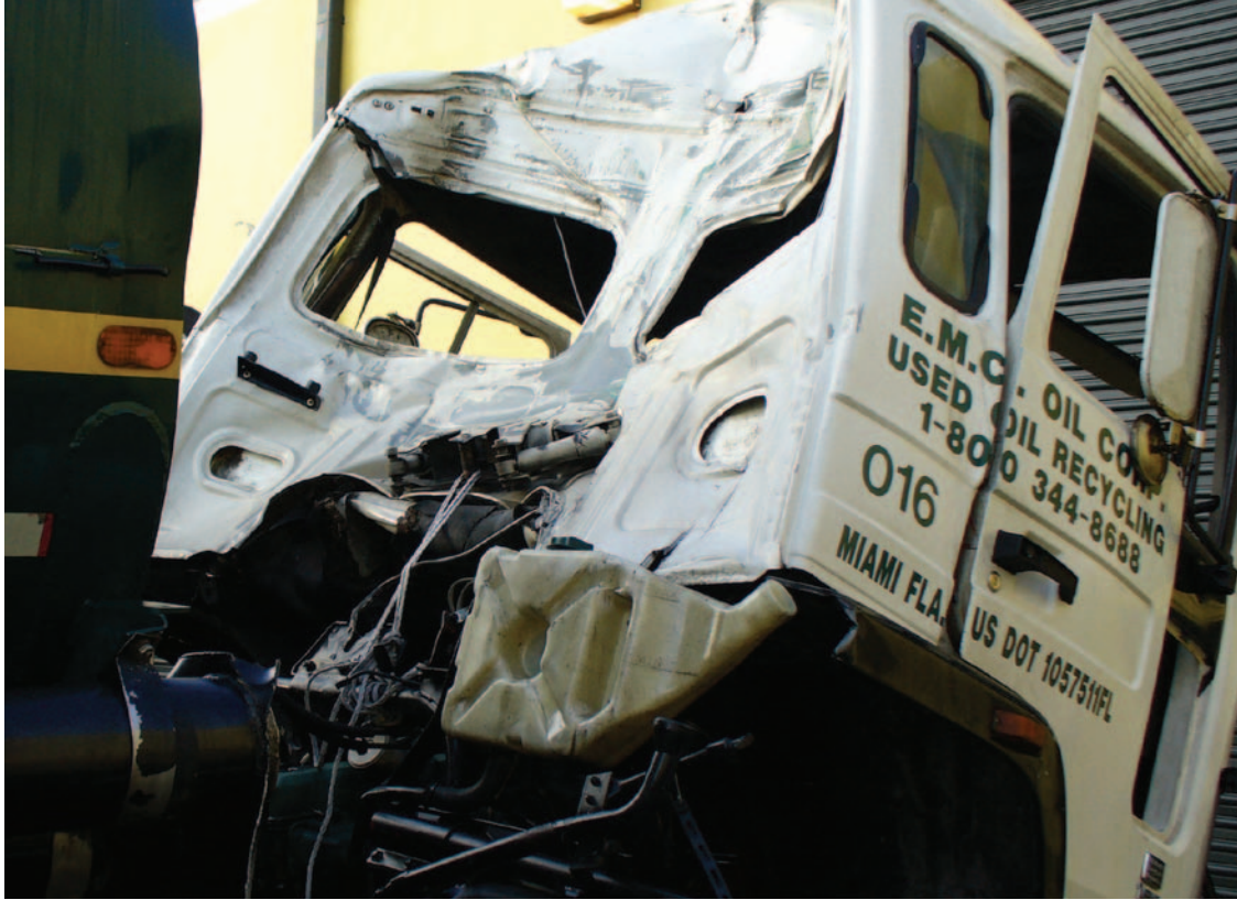
Damage to an oil tanker sustained from the December 2, 2008, explosion at EMC Used Oil Corporation.
